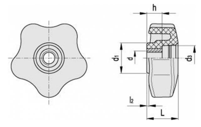
$\begin{array}{lll} D & = 74 \\ \text{d1} & = 26.5 \\ \text{d3} & = 19.5 \\ \text{dh} & = 10 \\ \text{h} & = 15 \\ \text{I2} & = 2 \\ \text{L} & = 24.5 \\ \text{Weight in (g)} = 48 \end{array}$
